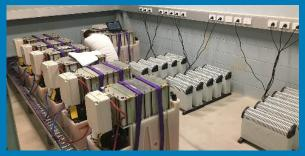
Figure 6. Zinc-bromine flow batteries in a performance testing lab. Source: Simon Hackett
