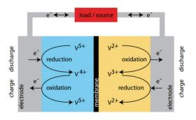
Figure 3. Vanadium redox flow battery charge and discharge process. Source: CDN
