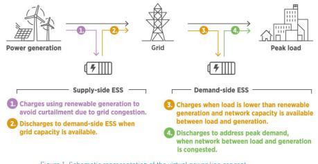
Figure 1: Schematic representation of the virtual power line concept Source: IRENA
