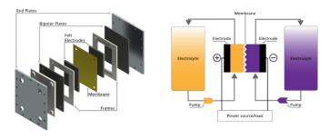
Figure 2. Exploded view and general schematic of a flow battery. Source: FlowCamp
