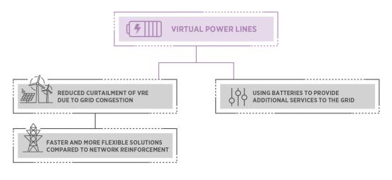
Figure 2: Contribution of virtual power lines to integrate variable renewable energy Source: IRENA
